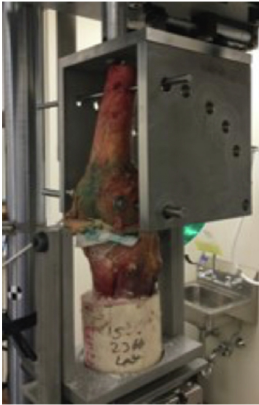
Fig 3. Final mounted specimen with TekScan sensors in place with combined apparatus to appropriately control various forces to evaluate tibiofemoral contact forces.
