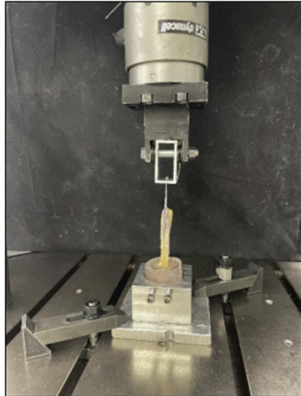
**Fig 1.** Testing set-up on the dynamic tensile testing machine.
